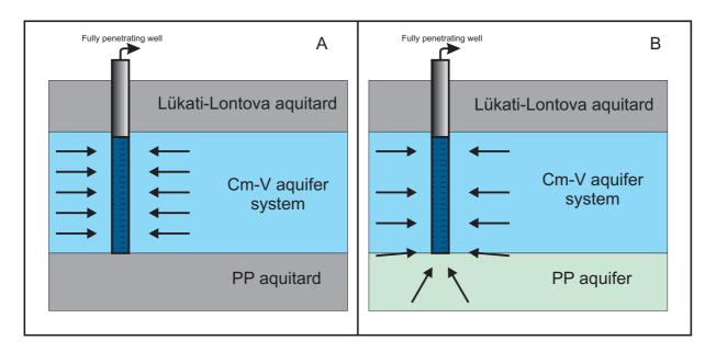
**Fig. 1.** Fully penetrating well in the Cambrian–Vendian aquifer system. Groundwater inflow to the well: (A) considering the PP layer as an aquitard, (B) considering the PP layer as an aquifer.
