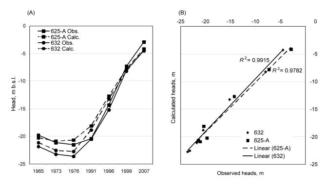
Fig. 4. The results of calibrations. (A) Observed and calculated heads during the calibration years. (B) Correlation between the observed and calculated values.
