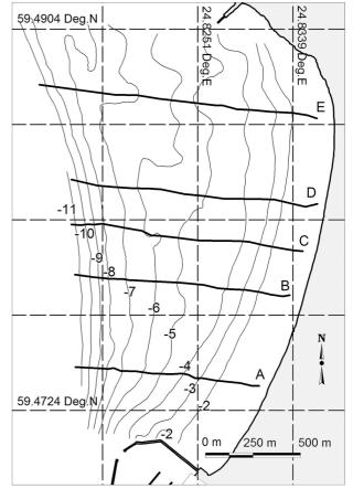
**Fig. 11.** Bathymetry of the nearshore of Pirita Beach according to the water depth survey in April 2006. The water depth along profiles A–E is given in Fig. 12. The coastline is shown based on the digital 1:50 000 Estonian Base Map from the Estonian Land Board (www.maaamet.ee).
