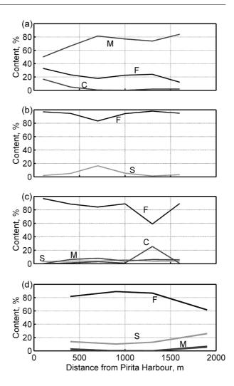
**Fig. 15.** Properties of different grain size fractions interpolated from sediment samples: (a) along the coastline, (b) along the 2-m isobath, (c) along the 5-m isobath, and (d) along the 10-m isobath. The letter C stands for coarse sand, M for medium sand, F for fine sand, and S for the fraction with the grain size <0.063 mm. Refer to Fig. 9 for sample locations.
