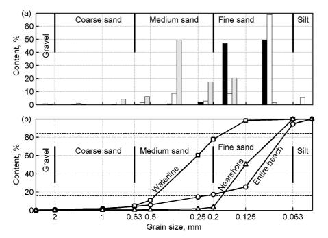
**Fig. 10.** (a) The content and (b) the cumulative distribution of different grain size fractions at Pirita based on samples collected in 2005 and 2007. Refer to Fig. 9 for sample locations. The averaged properties are shown for sand along the waterline (grey bars, squares), in the area with a depth of ~1 m (nearshore in 2007, white bars, triangles), and for the entire beach (filled bars, circles). The horizontal dashed lines on panel (b) represent 16% and 84% of the sand mass.
