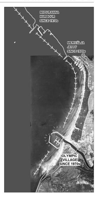
**Fig. 5.** Basic sediment transport and supply processes at Pirita Beach in natural conditions: natural longshore transport (arrows along a continuous line), river-induced sand supply (small triangles) and scarp erosion at the northern end of the beach (bold arrows). The contemporary coastline (white line) is given according to 1:50 000 Estonian Base Map from the Estonian Land Board (www.maaamet.ee). The background aerial photo used by the courtesy of the Estonian Land Board.
