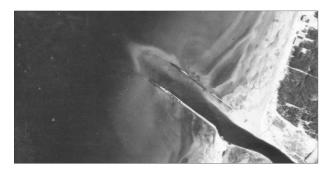
**Fig. 6.** The Pirita River mouth in 1951 (detail of the photo in Fig. 5) illustrating the joint effect of groins along the river coasts and the river flow on the formation of the sand bar at the end of the groins.
