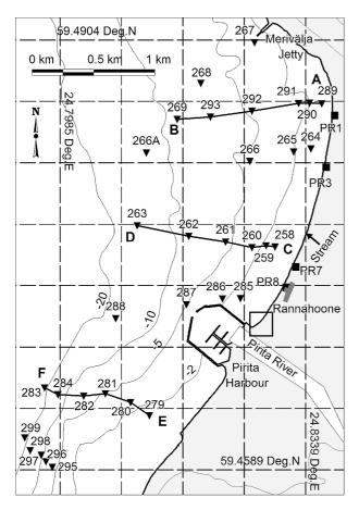
**Fig. 3.** Location of samples used for the construction of cross-sections A–B, C–D, and E–F (Fig. 4) of the upper sediment layers in Lutt (1992), Lutt & Tammik (1992), and for the analysis of properties of bottom sediments. Filled squares PR1, PR3, PR7, and PR8 denote the starting points of beach profiles 1, 3, 7, and 8 in Fig. 7. The box between Rannahoone and Pirita Harbour indicates the area represented in Fig. 8.
