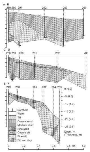
**Fig. 4.** Geological cross-sections of the beach area. Adapted from Lutt (1992) using the following nomenclature of the grain size: below 0.01 mm – silt and clay; 0.01–0.05 mm – fine silt; 0.05–0.1 mm – coarse silt; 0.1–0.25 mm – fine sand; 0.25–0.5 mm – medium sand; 0.5–1.0 mm – coarse sand. Location of the boreholes is given in Fig. 3.
