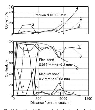
**Fig. 14.** Properties of different grain size fractions along beach profiles 1–6 in Fig. 9: (a) silt, (b) fine and medium sand.
