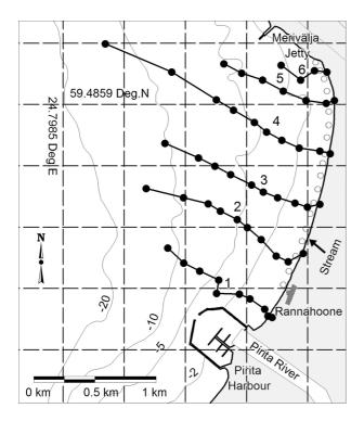
**Fig. 9.** Sampling points of bottom sediments at Pirita in 2005 (profiles 1–6) and 2007 (points in the nearshore, marked by empty circles). Isobaths of –2, –5, –10, and –20 m are shown based on the digital 1:50 000 Estonian Base Map from the Estonian Land Board (www.maaamet.ee).
