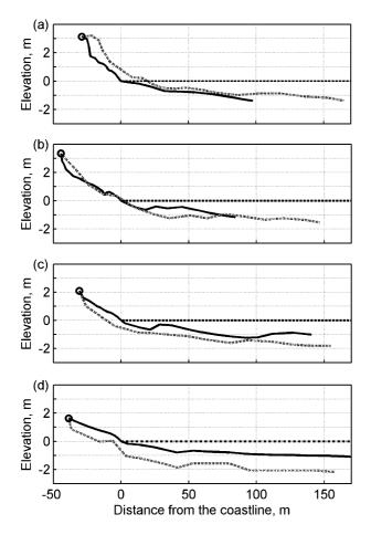
**Fig. 7.** Beach profiles 1 (a), 3 (b), 7 (c), and 8 (d) at Pirita on 9 Sept. 2003 (solid lines) and in 1994 (dashed lines) based on data from Suuroja et al. (2004). The profiles begin from the coastal scarp marked by a circle; refer to Fig. 3 for their location. The horizontal dashed line shows the mean water level
