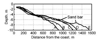
**Fig. 12.** Beach profiles (A–E) from the middle of the equilibrium profile to the 10 m isobath in April 2006. Refer to Fig. 11 for the location of profiles.
