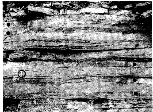
Fig. 6. Vertical distribution of rock types in a shale-poor, thin-bedded package showing predominance of arenites and siltites (light-grey layers). Layers of hard marlstones are denoted with black dot. Middle part of landslide scarp. Scale, 2 cm long, encircled
