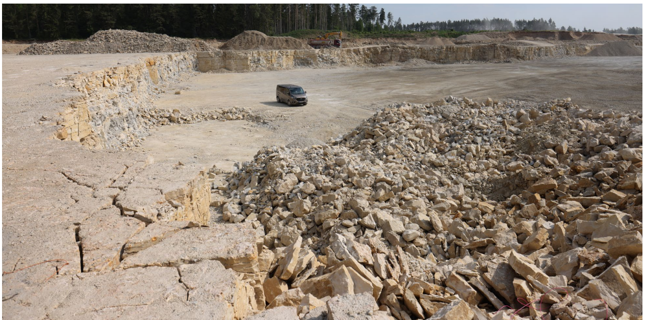
Fig. 20.2. Overview of the Sutlema quarry, showing mining of the Saunja limestone (carbonate mudstone), Nabala Regional Stage, Mid-Katian. Photo: Olle Hints, 2022.
