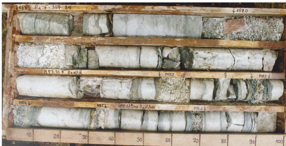
**Fig. 12.1.** Männamaa F-367 core box No 34, showing a series of Sandbian K-bentonites with the Kahula Formation, including the infamous Kinnekulle Bed, which marks the base of the Keila Regional Stage. Photo from the Estonian Land Board database.
