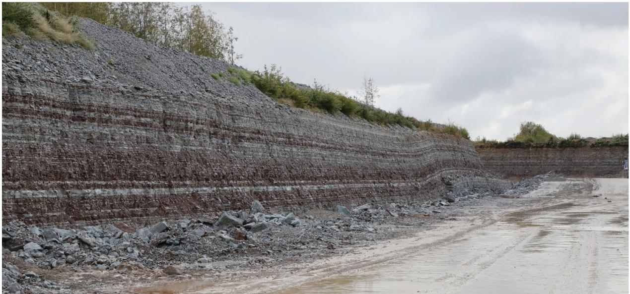
**Fig. 9.2.** Oil shale succession in the Põhja-Kiviõli II open-pit mine. Photo: Gennadi Baranov, 2019.
