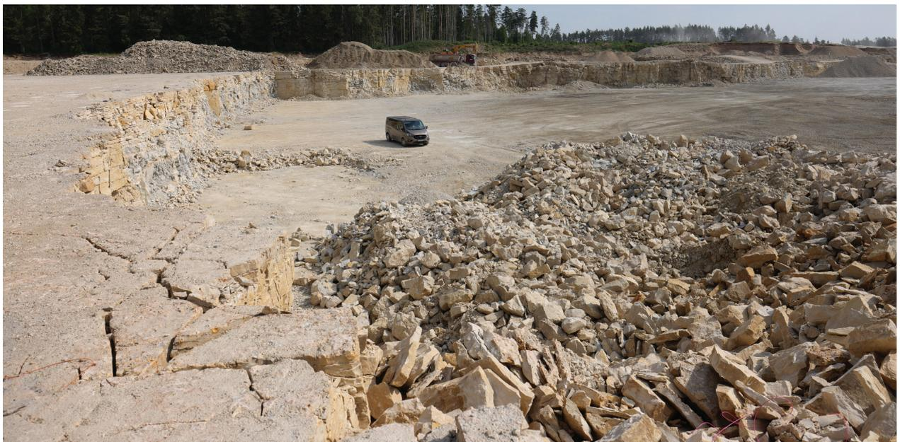
**Fig. 7.2.** Overview of the Sutlema quarry, showing mining of the Saunja limestone (carbonate mudstone), Nabala Regional Stage, Mid-Katian. Photo: Olle Hints, 2022.
