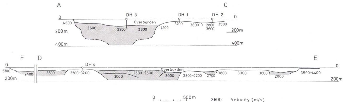
Fig. 6. Seismic profiles from the Söderfjärden structure
