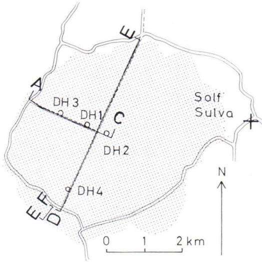
Fig. 4. Location of the seismic profiles and diamond drill holes.
