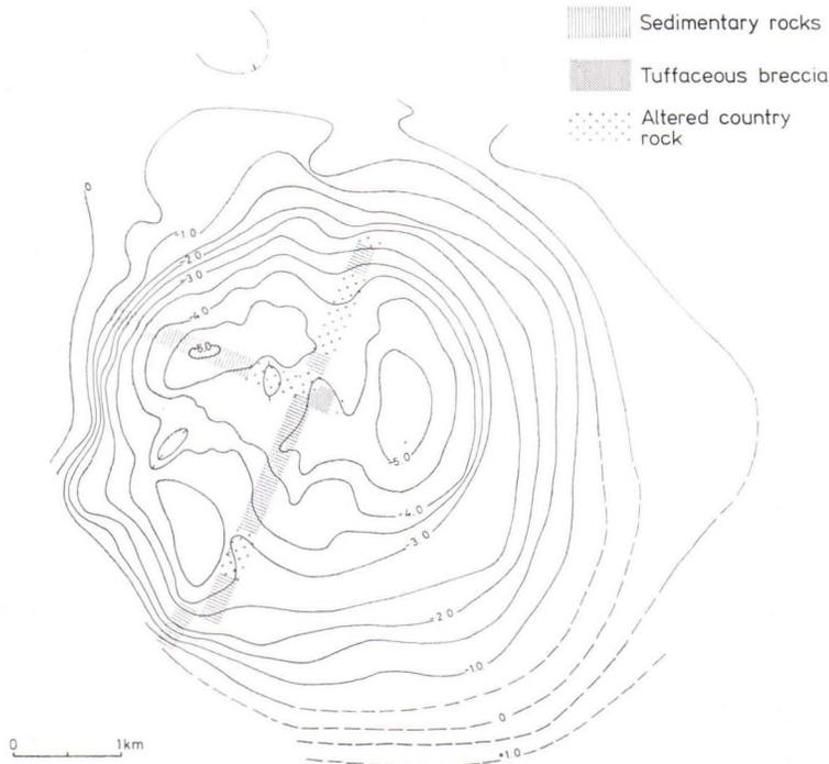
Fig. 10. Seismically determined distribution of the rocks within part of the Söderfjärden depression
