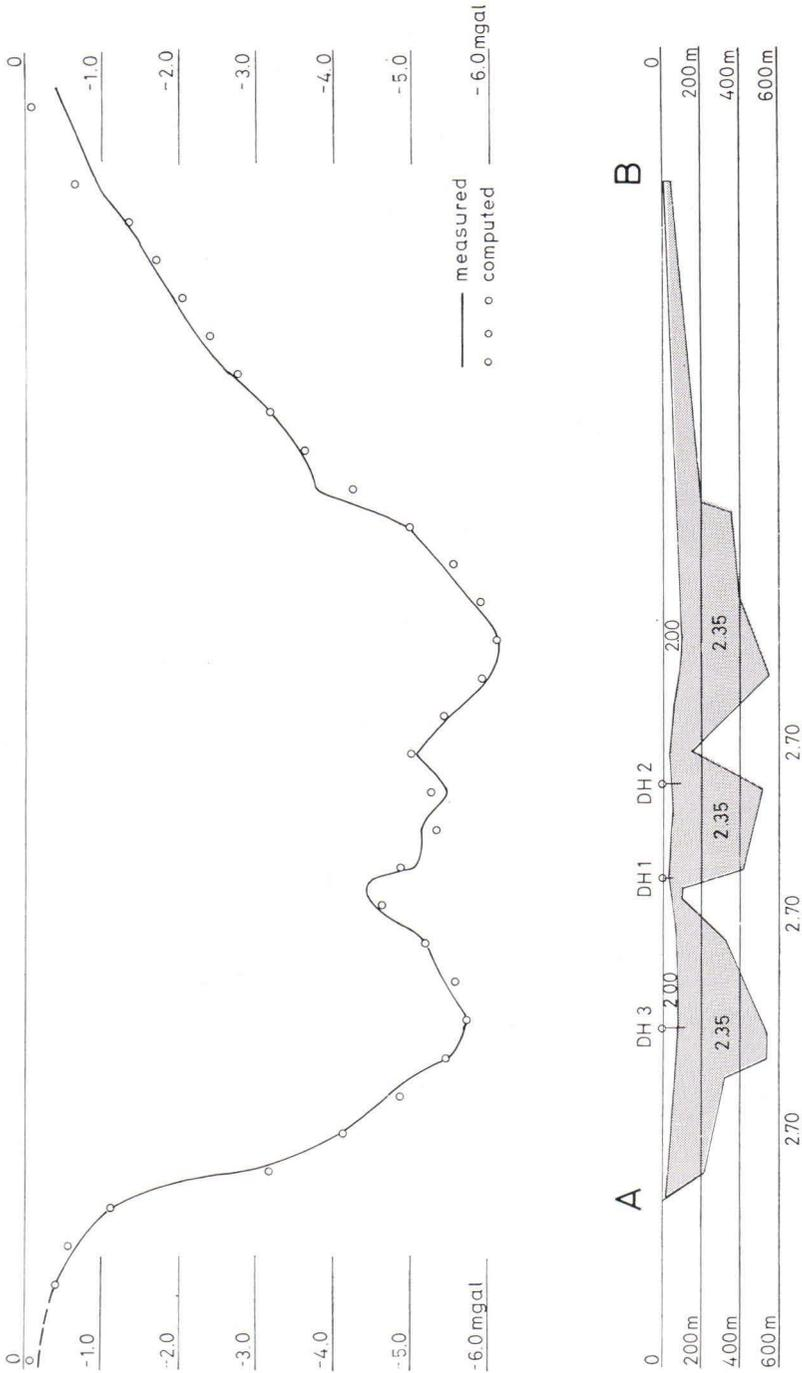
Fig. 9. Gravity model of the Söderfjärden structure.
