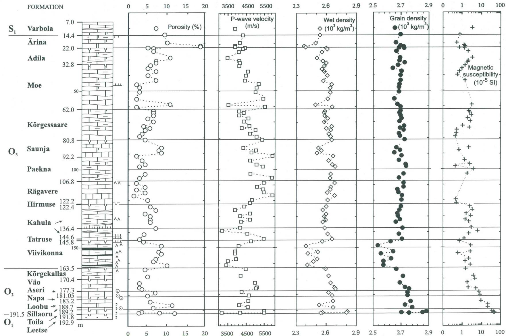
Fig. 12. Physical properties of the Kerguta (565) core. O<sub>1</sub> - Lower Ordovician; O<sub>2</sub> - Middle Ordovician; O<sub>3</sub> - Upper Ordovician; S<sub>1</sub> - Llandovery. Refer to Appendix 1 for lithology and distribution of the regional stages.
