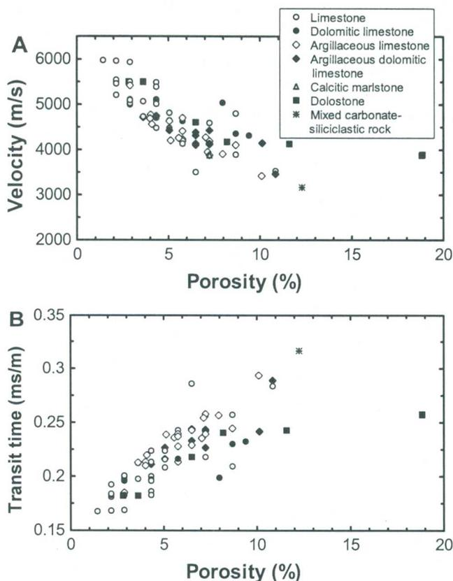
Fig. 13. (A) P-wave velocity versus porosity. Correlation coefficient  $R = -0.87$  for primary rocks (limestones, argillaceous limestones and calcitic marlstones),  $R = -0.67$  for dolomitized rocks (dolostones, dolomitic limestones, argillaceous dolomitic limestones and dolomitic marlstones).
