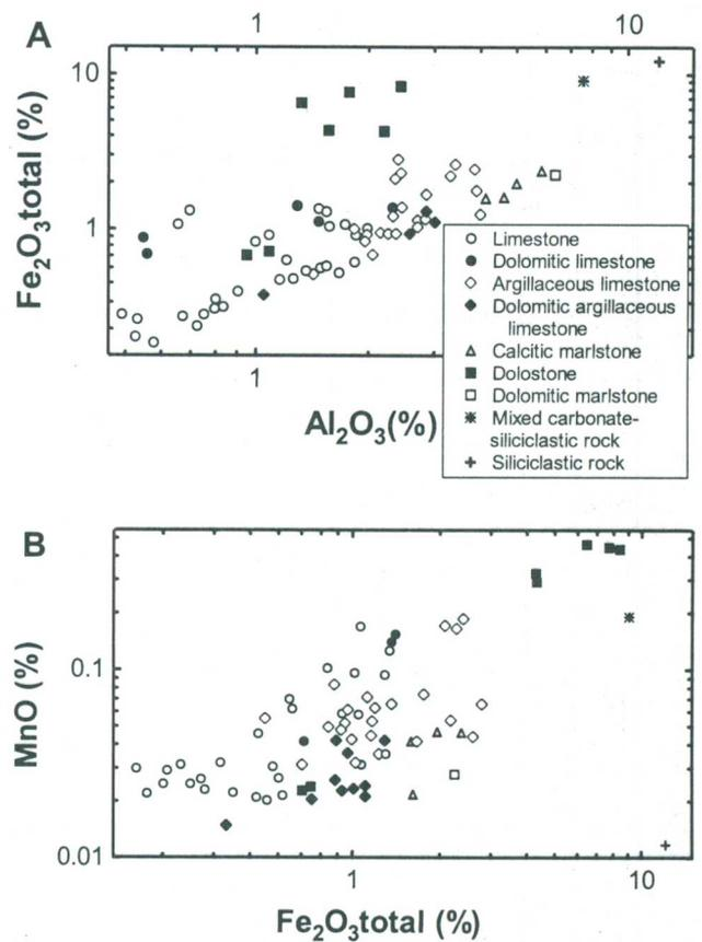
Fig. 9. (A) Total iron content versus  $\text{Al}_2\text{O}_3$  content measured by XRF analysis. Correlation coefficient  $R = 0.77$  for all samples except for the dolostones.
