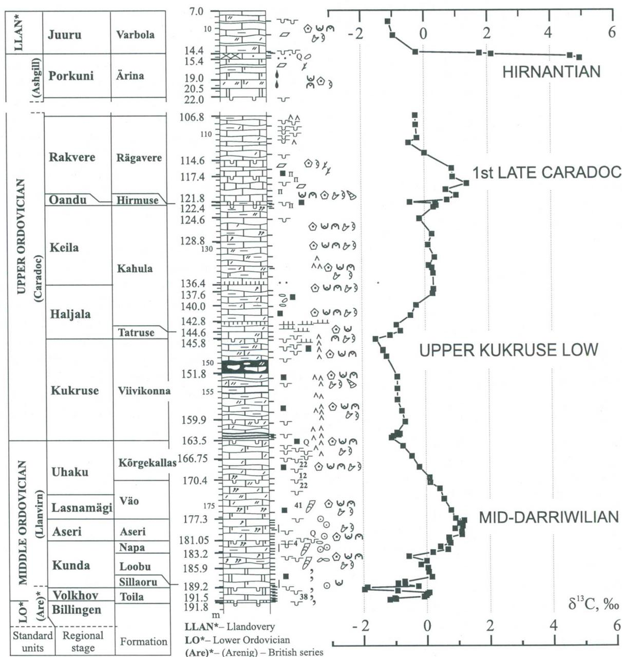
Fig. 4. The Ordovician and lowermost Silurian bulk carbonate carbon stable isotope profile of the Kerguta (565) core. Refer to Appendix 1 for lithology and Appendix 12 for sample depths. Sampling points are marked on the right side of the column.
