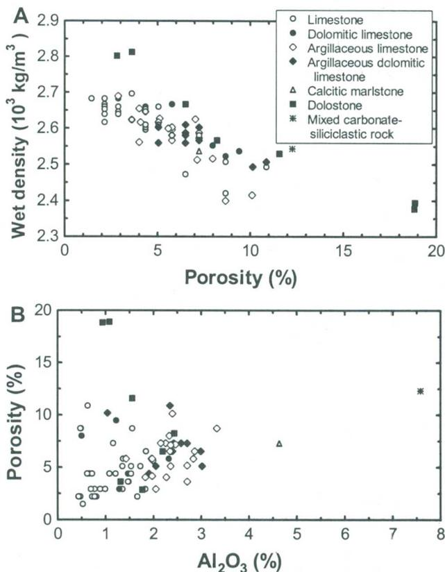
Fig. 11. (A) Wet density versus porosity. Correlation coefficient  $R = -0.80$  for primary rocks (limestones, argillaceous limestones and calcitic marlstones),  $R = -0.87$  for dolomitized rocks (dolostones, dolomitic limestones, argillaceous dolomitic limestones and dolomitic marlstones).
