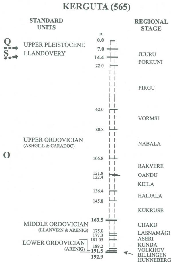
Fig. 2. Generalized stratigraphy of the Kerguta (565) core.
