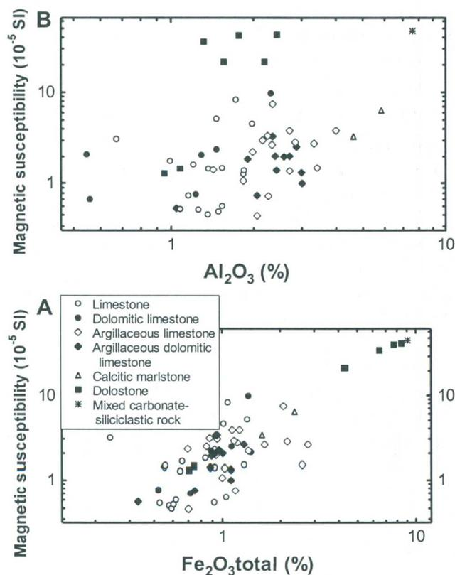
Fig. 14. (A) Magnetic susceptibility versus total iron content. Correlation coefficient  $R = 0.96$  for all rock samples. (B) Magnetic susceptibility versus  $Al_2O_3$  content.
