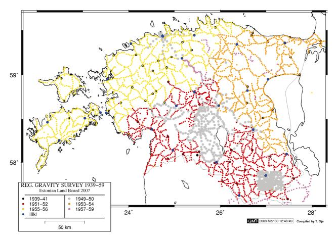
**Fig. 3.** Distribution of the 1949–58 gravity survey points. About 110 erroneous survey points were removed during the update of the Estonian Land Board database in 2007. The 1939–41 gravity points (altogether 101) are not used in the present study.
