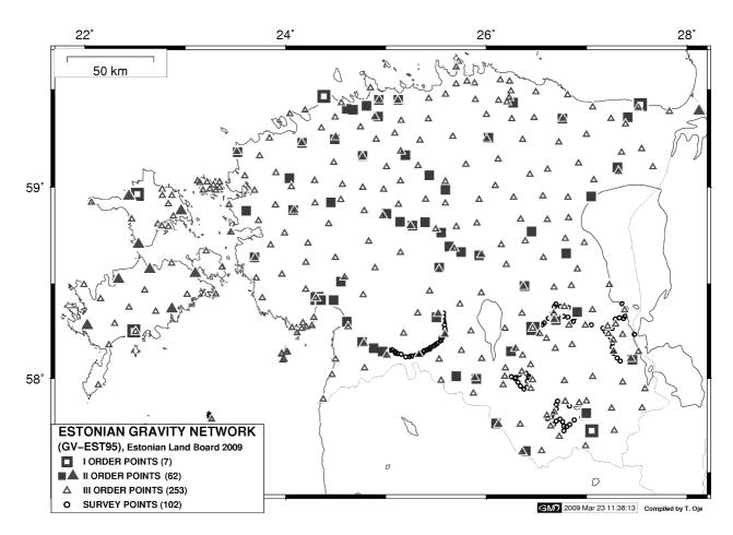
Fig. 2. Distribution of gravimetric control points used in the present study. The total number of control points is 424, comprising 322 national gravity network points and 102 Estonian Land Board precise gravity survey points.
