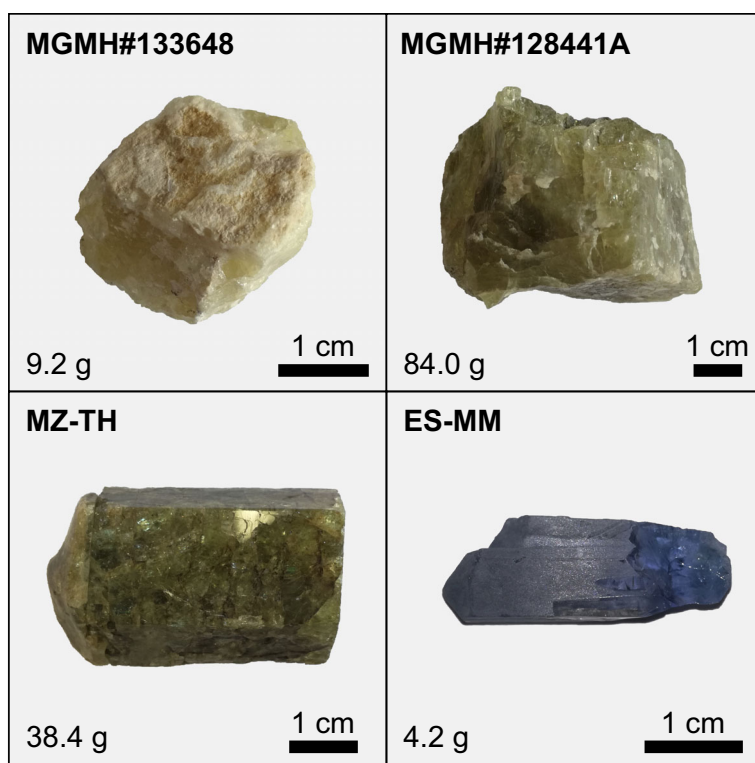
Figure 1. Photographs of the unprocessed apatite samples characterised in this study. Total masses of crushed apatite material produced after completion of mineral separation are given in the bottom left of each panel. The two specimens MGMH#133648 and MGMH#128441A have already been characterised for their chlorine isotope compositions by Wudarska et al. (2021).
