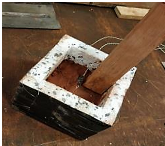
Fig. 3. Casting of the thermal block with thermocouples placed at varying depths.
