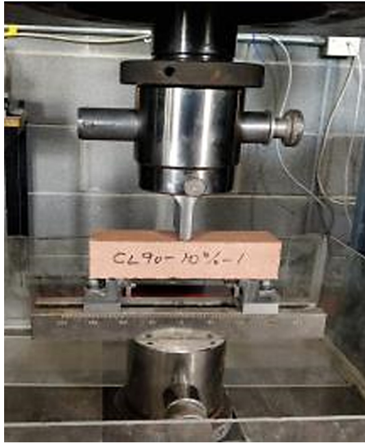
Fig. 2. Device assembly for the three-point flexural strength test showing a clay specimen stabilized with hydrated lime.
