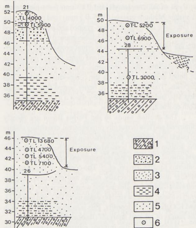
Fig. 105. Sections dated with TL method. For location of sections and boreholes see Fig. 104: 1 – till; 2 – glaciofluvial deposits; 3 – glaciolacustrine sand; 4 – glaciolacustrine silt; 5 – aeolian sand; 6 – location of dated samples (after Raukas & Hütt 1998).
