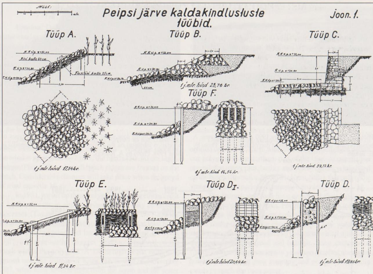
Fig. 89. Constructions that were recommended for the protection of the Peipsi coast at the end of the 1920s and in the beginning of the 1930s (after Vichmann 1929).
