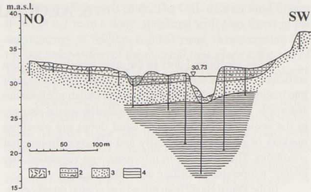
Fig. 103. Cross-section in the mouth of the Rannapungerja River (after Dzilna with complements of Miidel & Tavast 1981): 1 - peat; 2 - overbank deposits (silty sand with organic matter); 3 - channel deposits (sand); 4 - varved clay.
