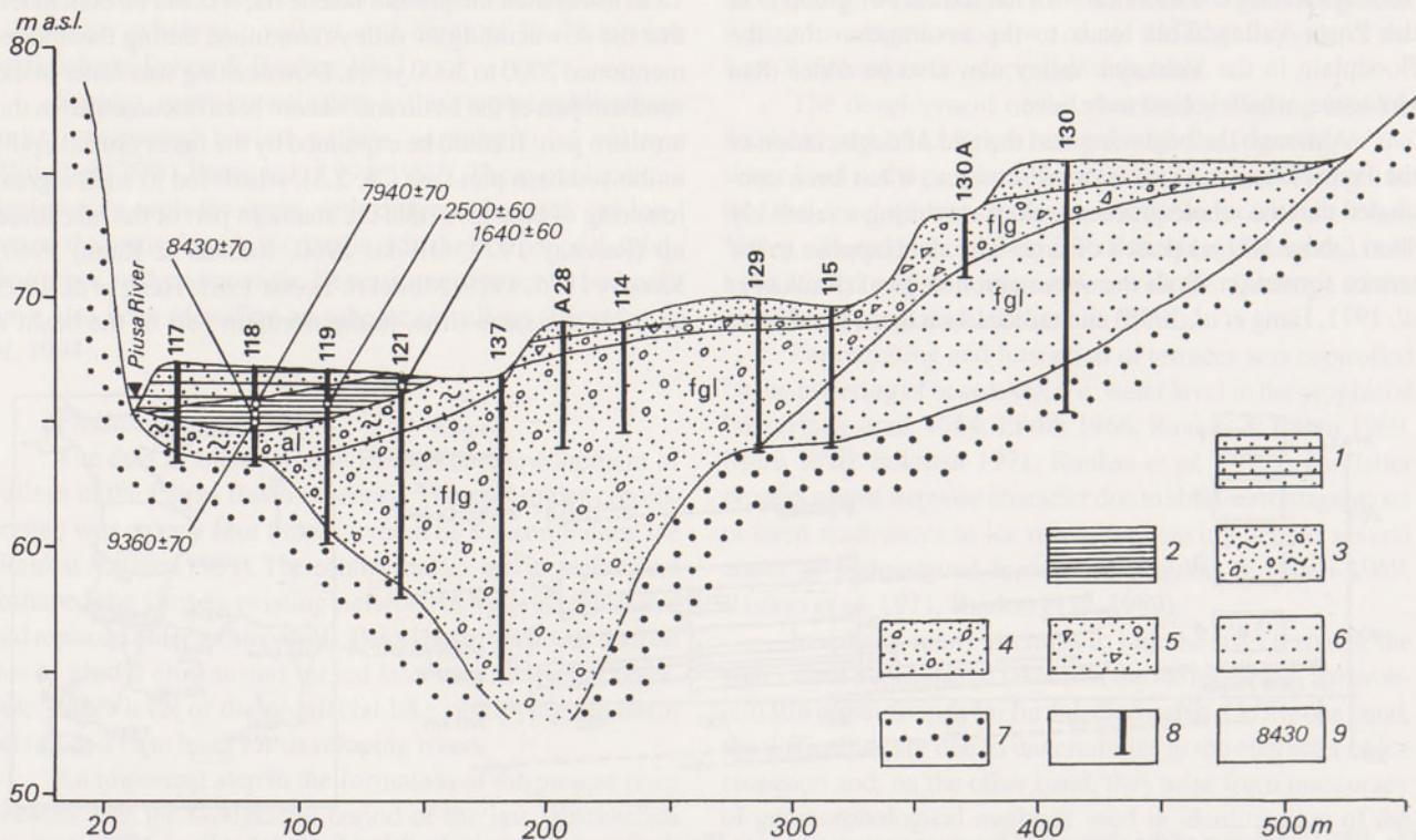
Fig. 101. Cross-section of the Piusa Valley near Härrma (after Hang 1995): 1 - overbank deposits; 2 - oxbow deposits; 3 - channel deposits; 4 - glaciofluvial sand and gravel; 5 - glaciofluvial gravel with pebbles; 6 - glaciolacustrine sand; 7 - terrigenous Devonian rocks; 8 - borehole; 9 -  $^{14}\text{C}$  datings (yr BP).
