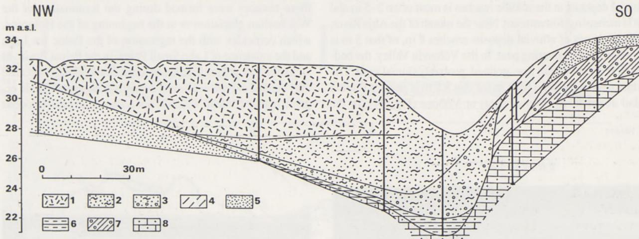
Fig. 93. Cross-section of the Ahja River, near Lääriste (after Pärna, with complements of Miidel & Tavast 1981): 1 - peat; 2 - sandy and 3 - gravelly river deposits with plant remnants; 4 - slope wash; 5 - glaciolacustrine sand; 6 - glaciolacustrine silt; 7 - till; 8 - Devonian sandstone.
