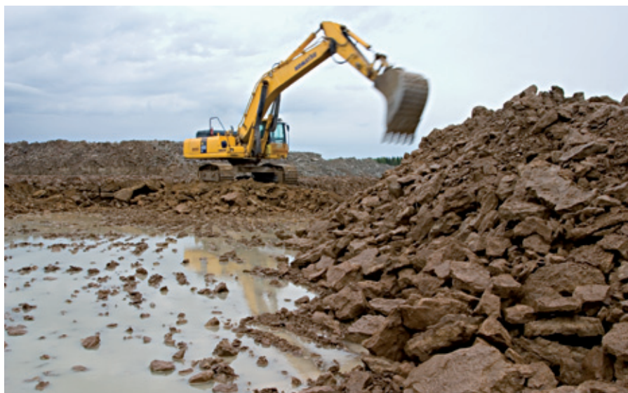
Oil shale mining in the Põhja-Kiviõli opencast: mining of D-F 1 oil shale sequence (above). Surface miner Wirtgen 2500 SM allows selective mining of oil shale seams B+C as well as a pure limestone interbed C/D (below)
