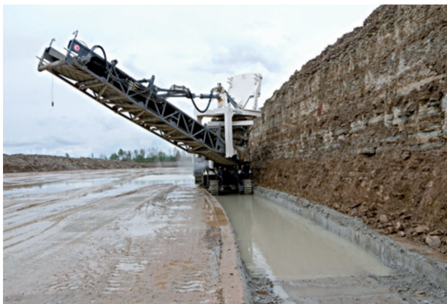
Oil shale mining in the Põhja-Kiviõli opencast: mining of D-F 1 oil shale sequence (above). Surface miner Wirtgen 2500 SM allows selective mining of oil shale seams B+C as well as a pure limestone interbed C/D (below)
