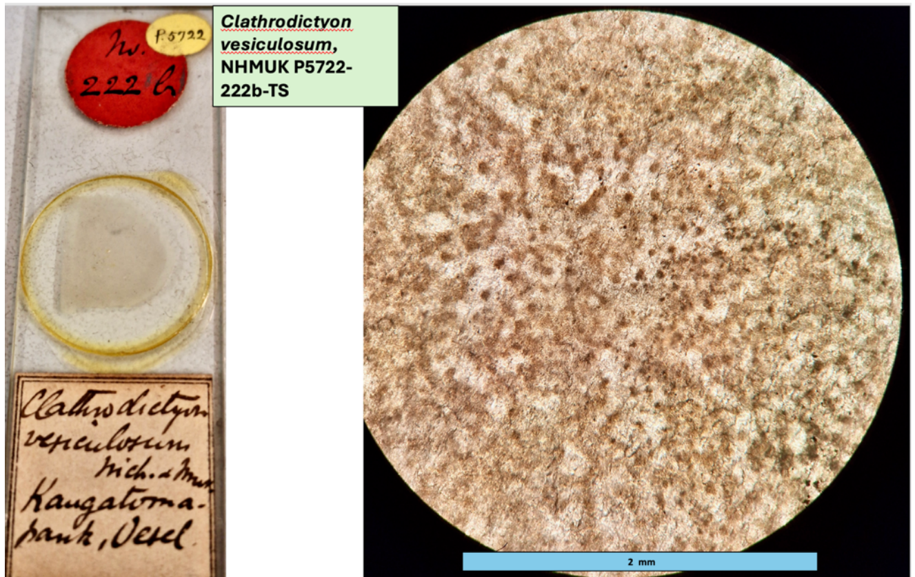
Fig. 4.2.6. TS of C. vesiculosum , with a skeletal structure that shows pillars consistent with C. vesiculosum in some areas. However, other areas may represent transverse cuts through the upper or lower parts of the zigzag structure seen in VS. Overall the structure more closely resembles Ecclimadictyon . Specimen NHMUK PI P5722-222.
