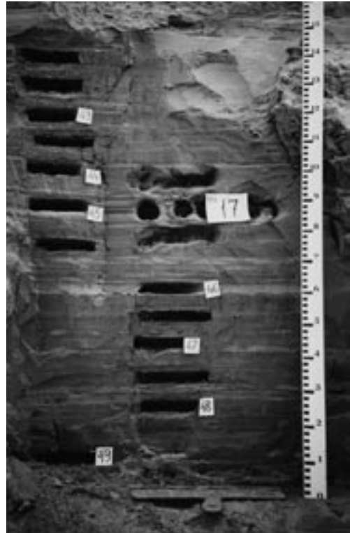
One of the Voka V3-03 section stripping showing the stratigraphy of the deposits and sampling points for pollen, diatom and luminescence (OSL) analyses. Photo by A. Molodkov.
