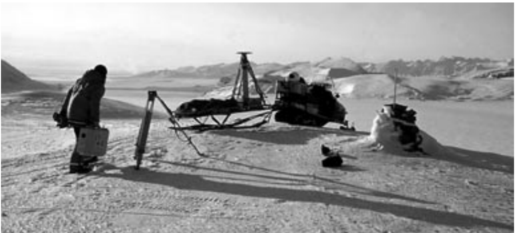
Growth of glaciers can best be measured using satellite positioning systems. In this photo, a high precision GPS is being calibrated by the “fixed point” at the top of Mount Annekammen, Svalbard (glacier Kongsvegen in the background). Photo by T. Martma.
