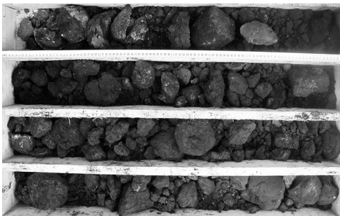
The core from the well drilled through the Kukruse waste landfill, which was examined for trace elements and organic compounds. Photo by G. Baranov.
