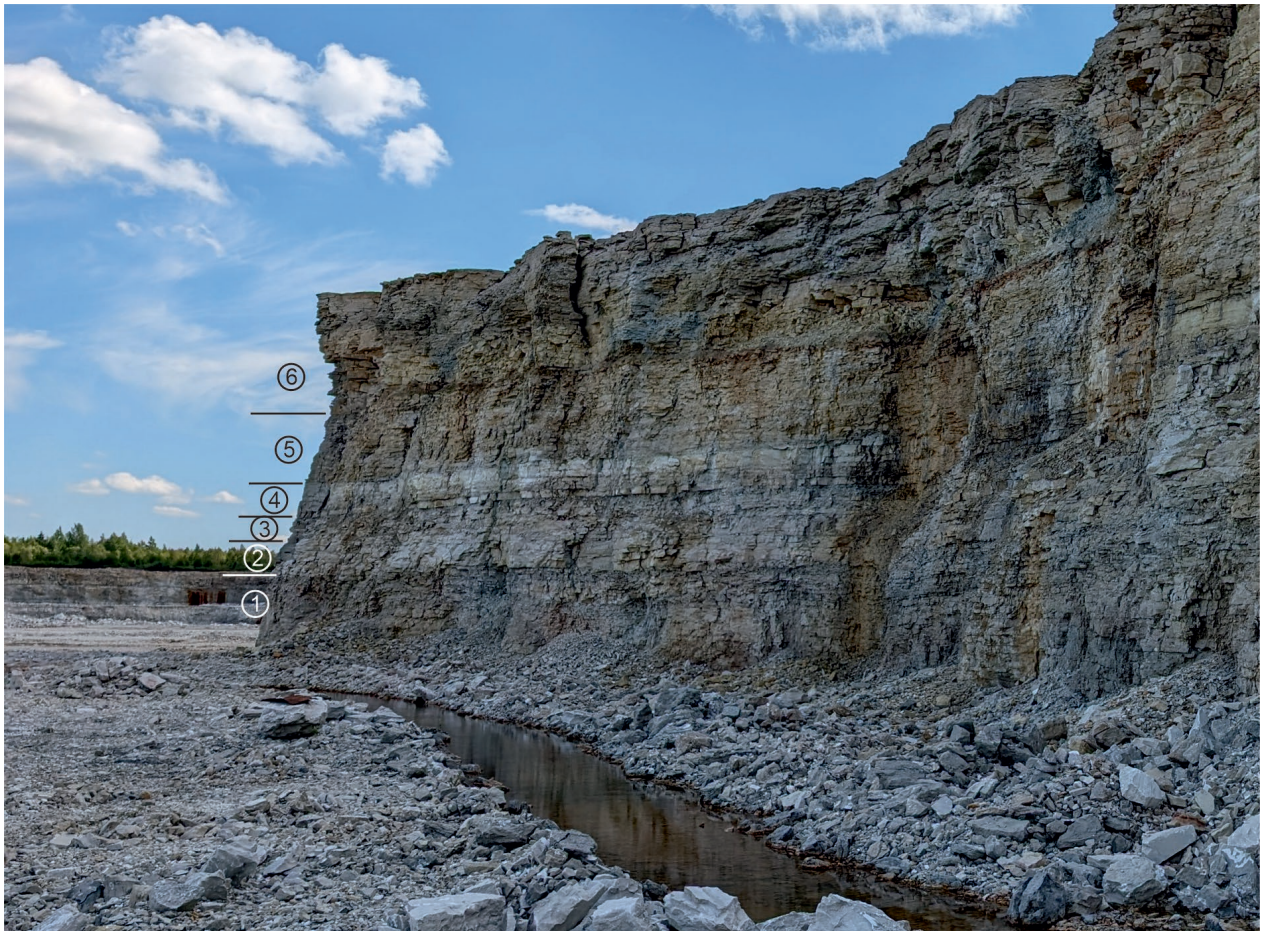
Fig. 2.1. The western wall of the Kalana quarry (height about 15 m). Beds 1–5, Jõgeva Beds. 1 – fine-grained limestone (packstone, grainstone) with marl intercalations, 2.4+ m; 2 – massive grainstone (“Kalana Marble”), 0.8–1.2 m; 3 – grainstone with marl intercalations, 1–2 m; 4 – massive grainstone (“Kalana Marble”), with a bed of thin laminated grainstone-marl at the base, 0.5–1.0 m; 5 – grainstone intercalating with argillaceous limestone (wackestone, packstone) and marl, 3 m. Bed 6 , Imavere Beds – argillaceous limestone and marl (wackestone, mudstone), 3.5+ m.
