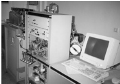
Finnigan MAT Delta E mass-spectrometer is used for isotope analysis of light elements.
