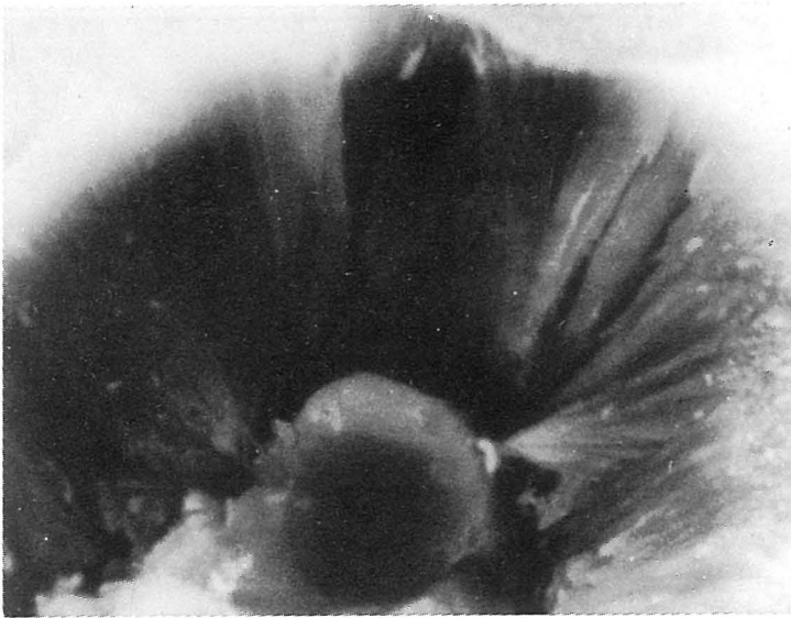
Fig. 6. A detail of Fig. 5. Radial crystallite aggregates of a phosphatic film. x7000.
