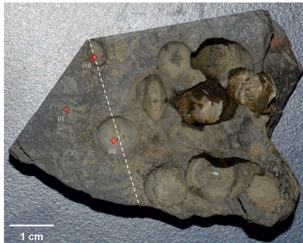
Figure 1. Photograph of a piece of siltstone collected from the middle reaches of the Kaladan River, western Myanmar, showing extensive pitting by Lignopholas fluminalis bivalves. The sample has been cut following the dashed line, and three locations were investigated by electron microscopy, namely (i) an area devoid of macroborings, the bottom of (ii) a large and (iii) a small macroboring, respectively.
